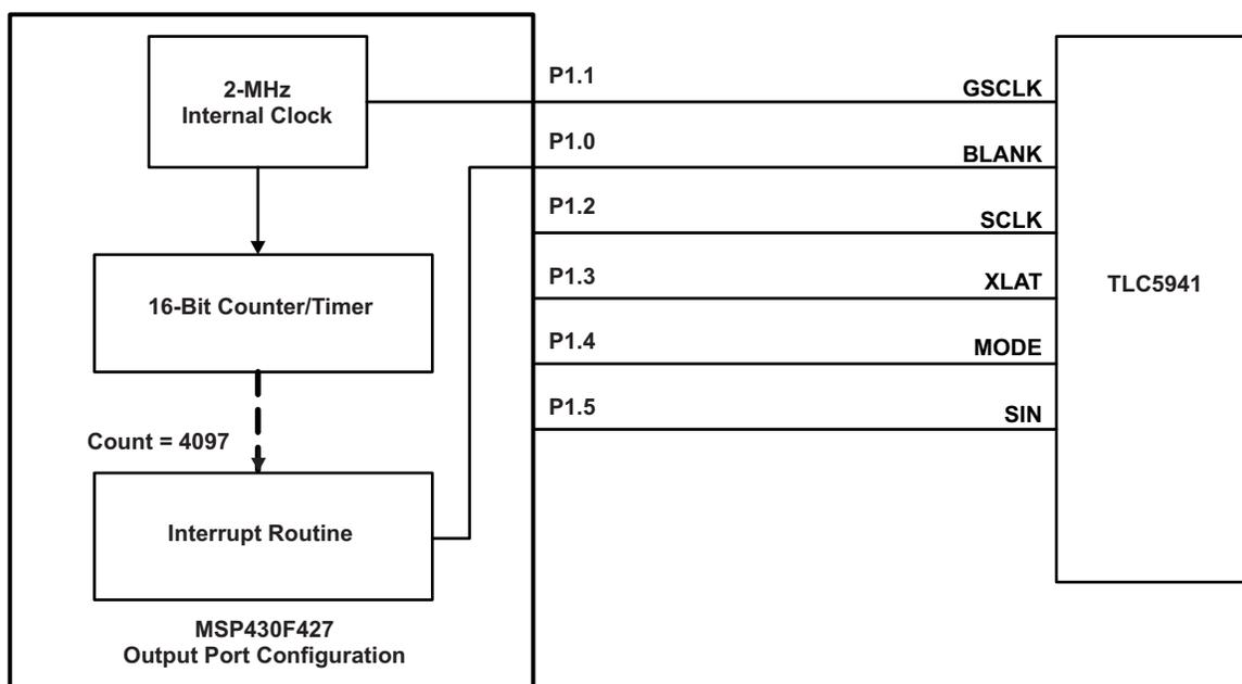
Figure 1. Simplified Block Diagram Of Clocking Scheme
